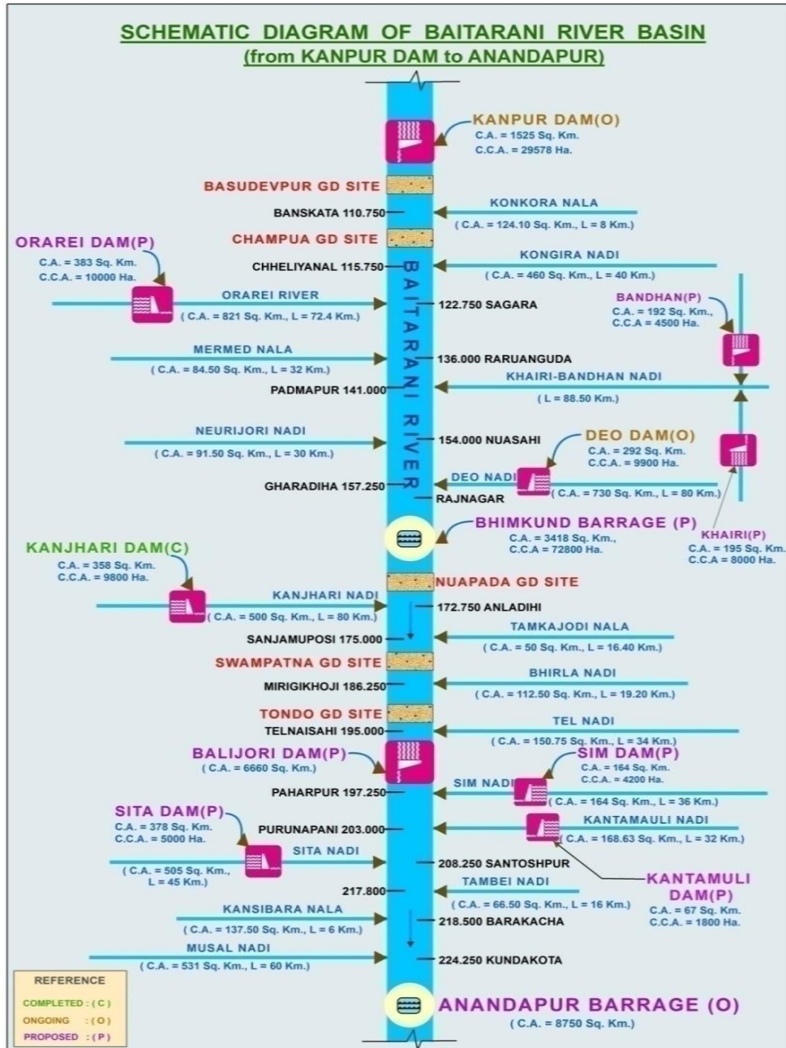
Figure 1.5: Schematic of Baitarni river from Kanupur to Anandpur
