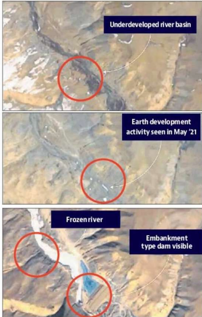
(From top) A satellite image before May 2021 shows no construction activity near the Mabja Zangbo river; but around May 2021, earth development activity can be seen near the river in Burang county of Tibet; latest images depict the obstruction of the river's path, the formation of a reservoir, and an embankment-type dam.
