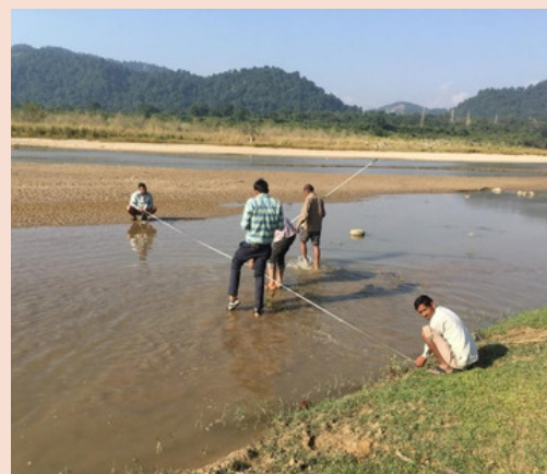
Cross-section survey work being carried out in Rāmgangā Basin for assessment of environmental flows under Indo-EU Joint Working Group
