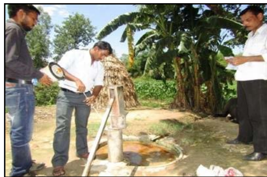
Ground Water Level measurement & Sample collection
