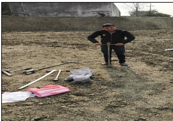
Infiltration Tests at pond bottom
