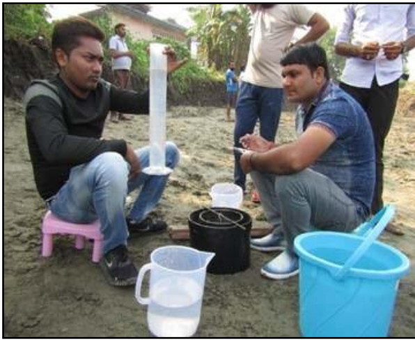
Infiltration test at pond bed
