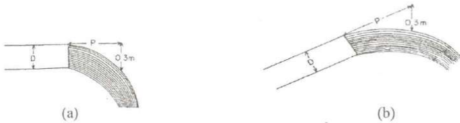
Fig. 3.1 Measurements for determining Discharge: (a) horizontal; and (b) inclined pipe
