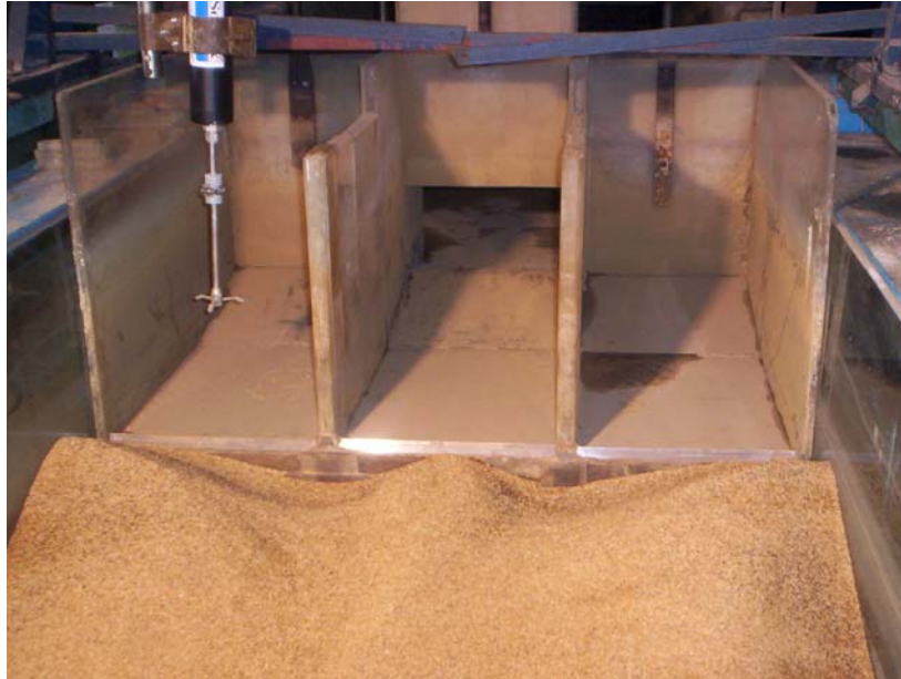
Fig. 4.4 Photograph after experimental run showing middle gate full open and two side gates closed with scour bed (0-F-0)
