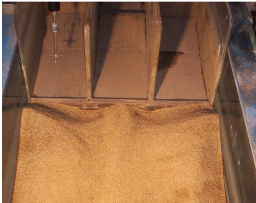
Fig. 4.4 Photograph after experimental run showing middle gate full open and two side gates closed with scour bed (0-F-0)
