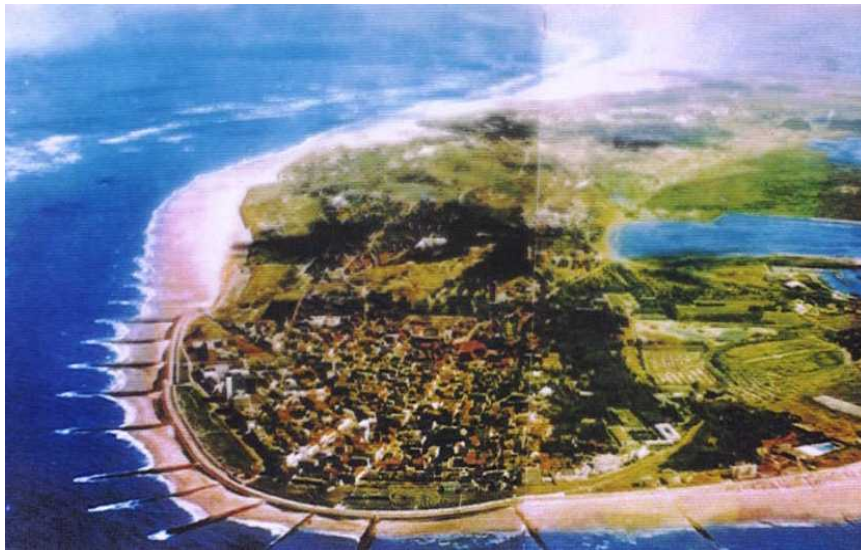
Photo.1.7 Groins field protecting the Island of Nordeney, Germany
