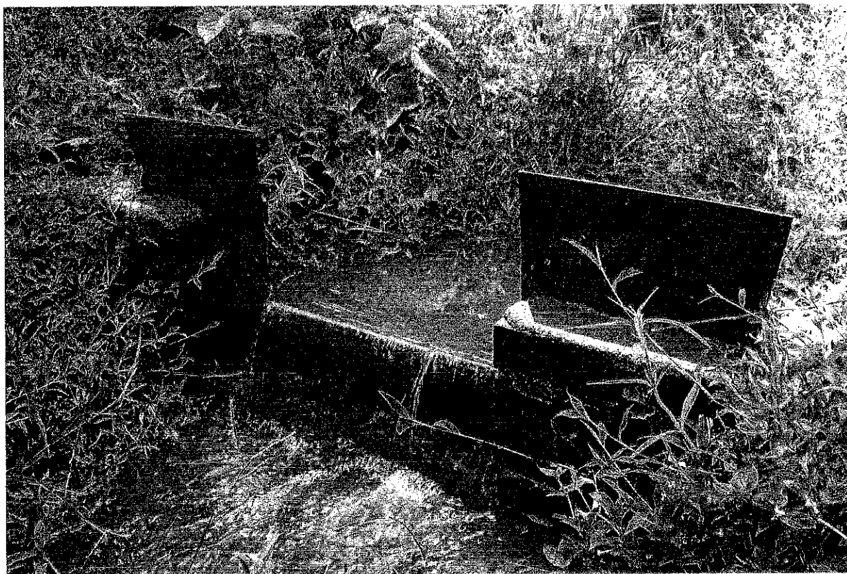
Plate 3 Rectangular weir installed for discharge measurement
