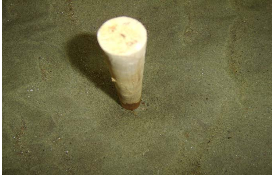
Picture 3.4: Scour details around pier after free-flow ( D = 3.2 cm)
