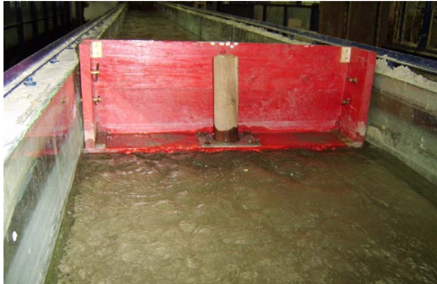
Picture 3.7: Experiment for D = 5.14 cm under pressure-flow conditions
