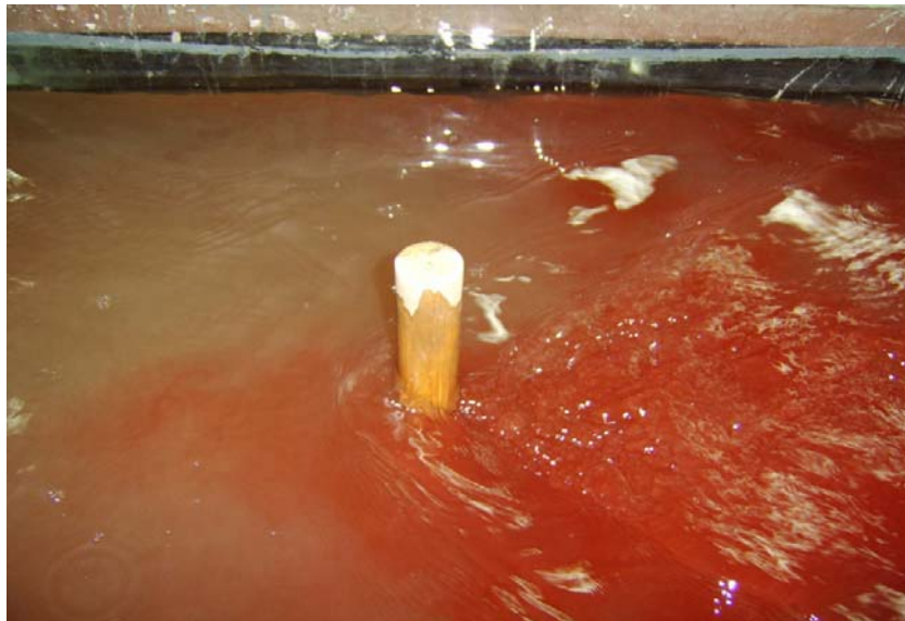
Picture 3.3: Experiment for D = 3.2 cm under free-flow conditions
