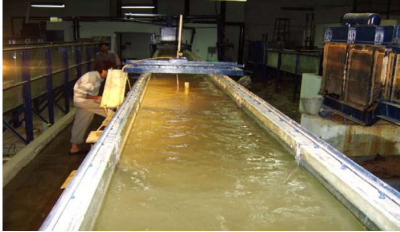
Picture 3.1: Glass-walled flume for carrying out experiments
