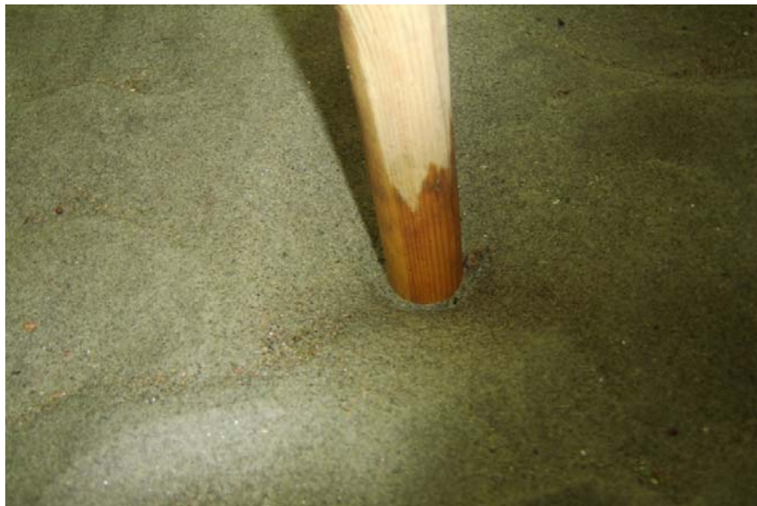
Picture 3.5: Scour details around pier after free-flow ( D = 3.2 cm)
