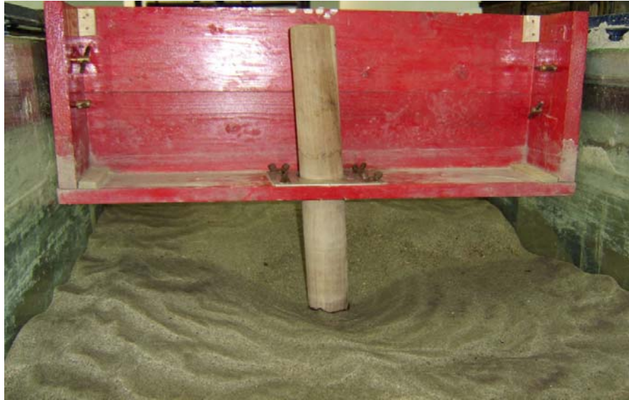
Picture 3.8: Scour details around pier after pressure-flow ( D = 5.14 cm)
