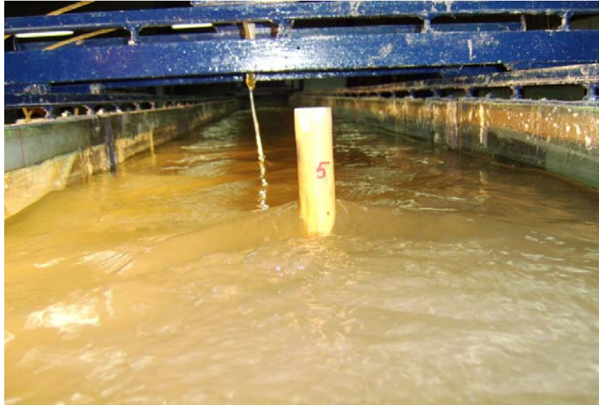
Picture 3.2: Experiment for D = 3.2 cm under free-flow conditions
