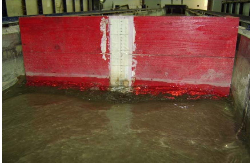
Picture 3.6: Experiment for D = 5.14 cm under pressure-flow conditions
