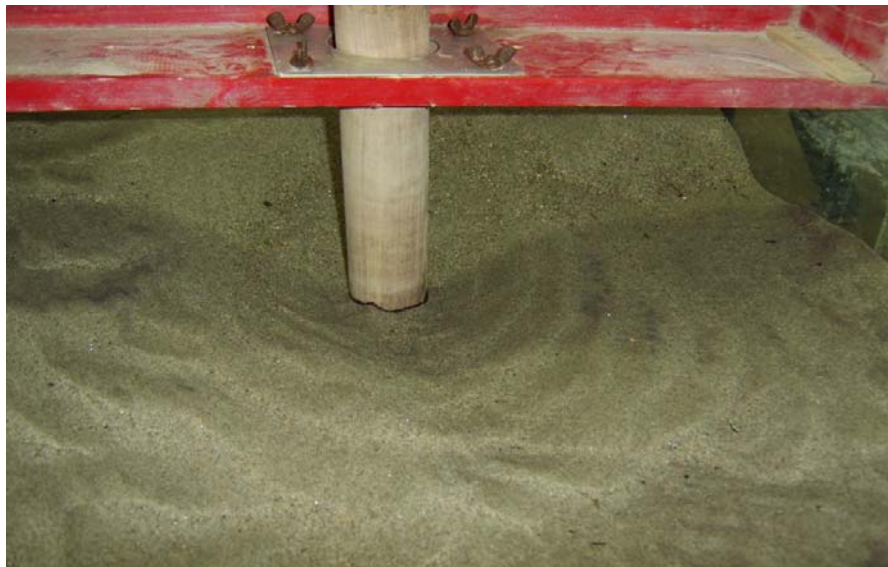
Picture 3.9: Scour details around pier after pressure-flow ( D = 5.14 cm)
