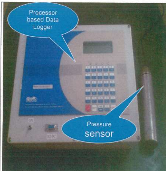
Fig.23: Micro Processor Based Data Logger with Pressure Sensor for Automatic Water Level Measurements
