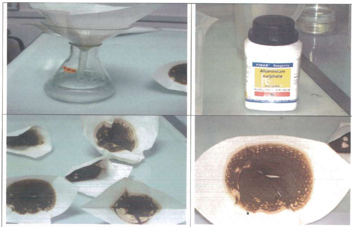
Fig.28: Laboratory Estimation of Sediment Yield from the Water Samples
