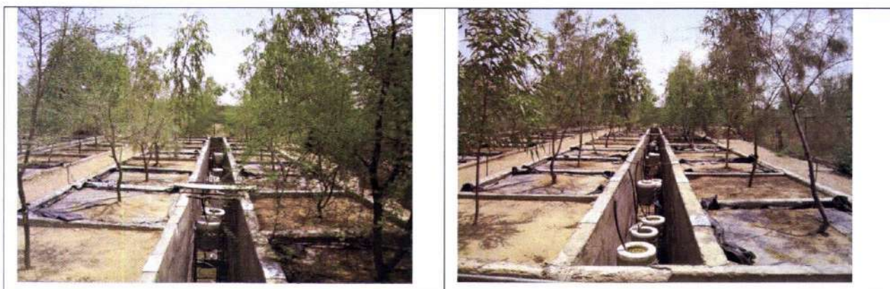
Lysimeters connected to 100 l tanks and polythene covering to check surface evaporation
