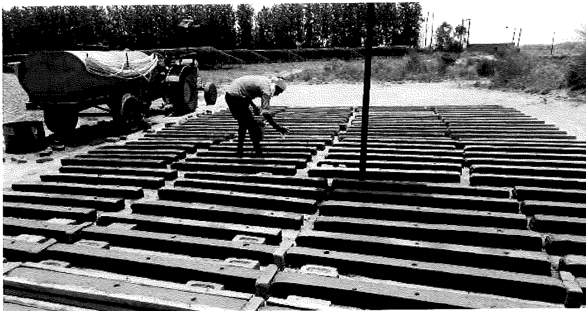
Figure 10.5 : Casting of RCC Jack
