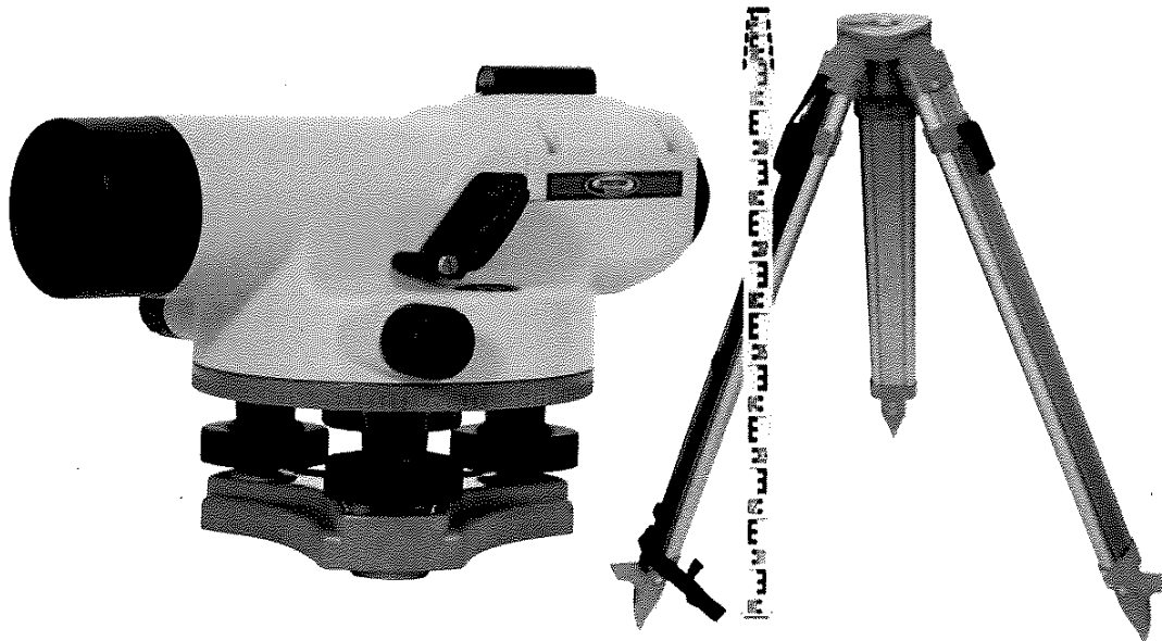
Figure 10.1 : Dumpy Level with Tripod stand and Staff
