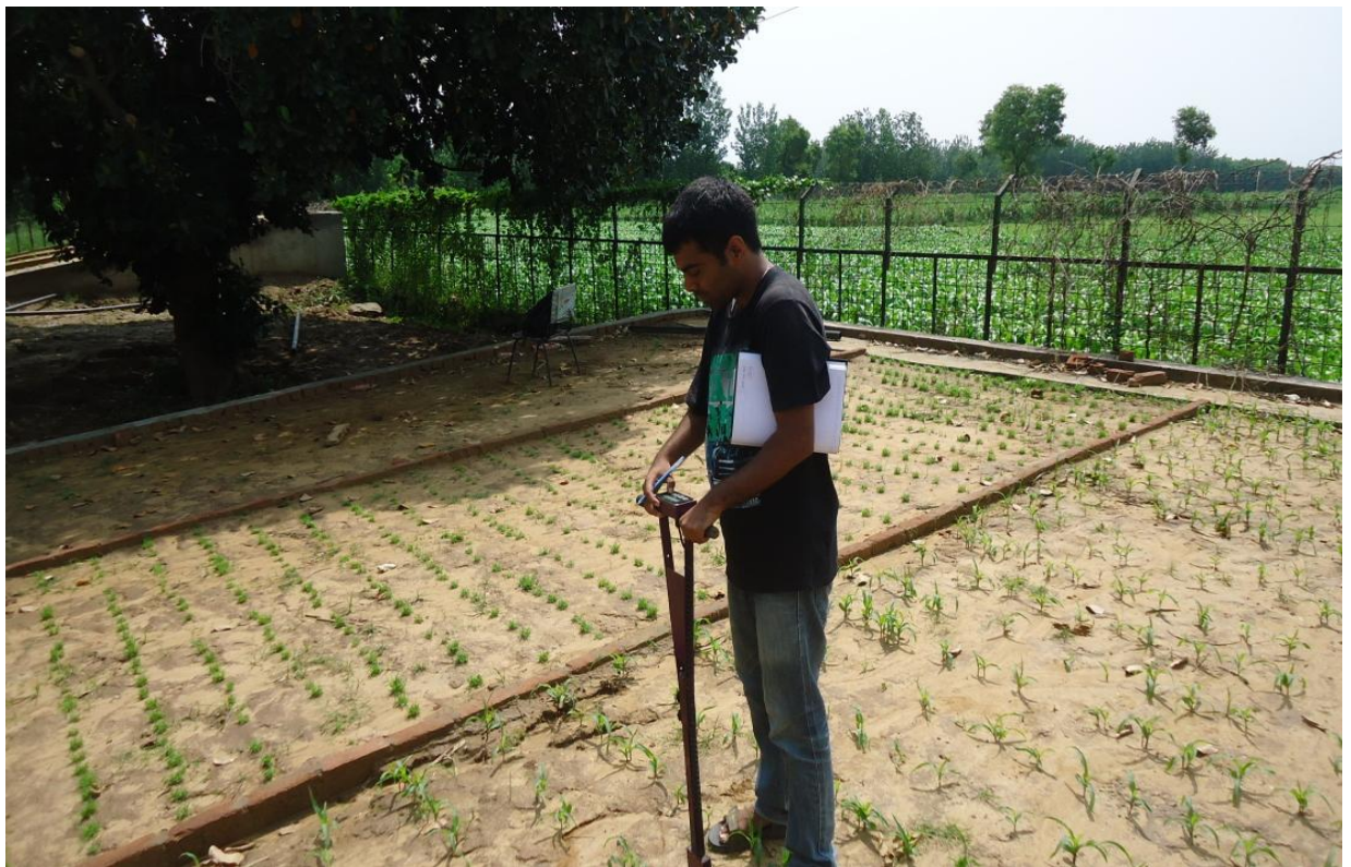
Figure 3.3b Measurement of soil Moisture Content ( \theta_o ) in maize plot during phase 2
