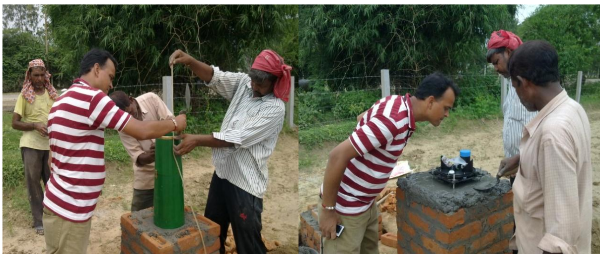
Figure 2.3a Setup of Ordinary Raingauge (ORG) and Self – Recording Raingauge (SRRG)
