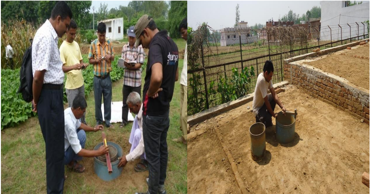
Figure 3.5a Installation of double ring infiltrometer during phase 1 & Phase 2
