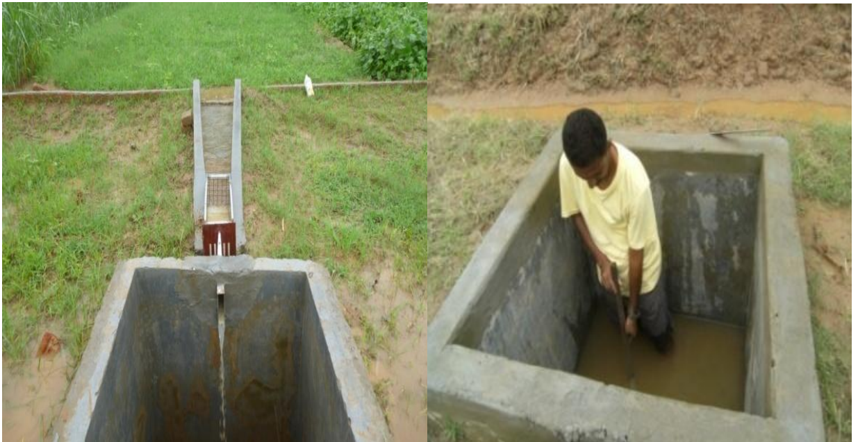
Figure 3.2 Runoff depth measurement by metallic measuring scale
