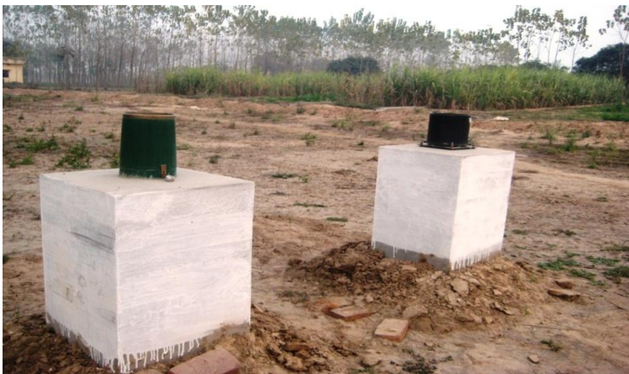
Figure 2.3b Finished ORG and SRRG ready for rainfall observation.
