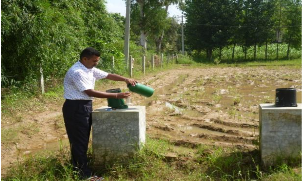
Figure 3.1 Rainfall measurement using non recording type raingauge
