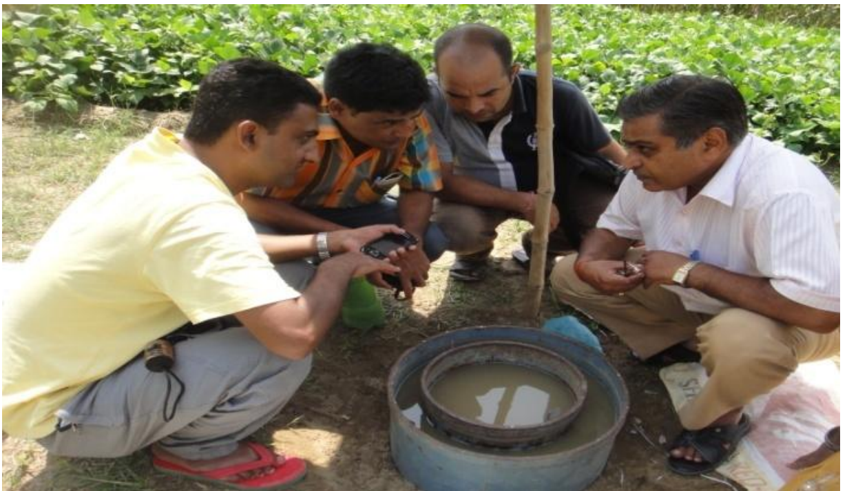
Figure 3.5b measuring the water level in double ring infiltrometer while conducting infiltration test during phase1
