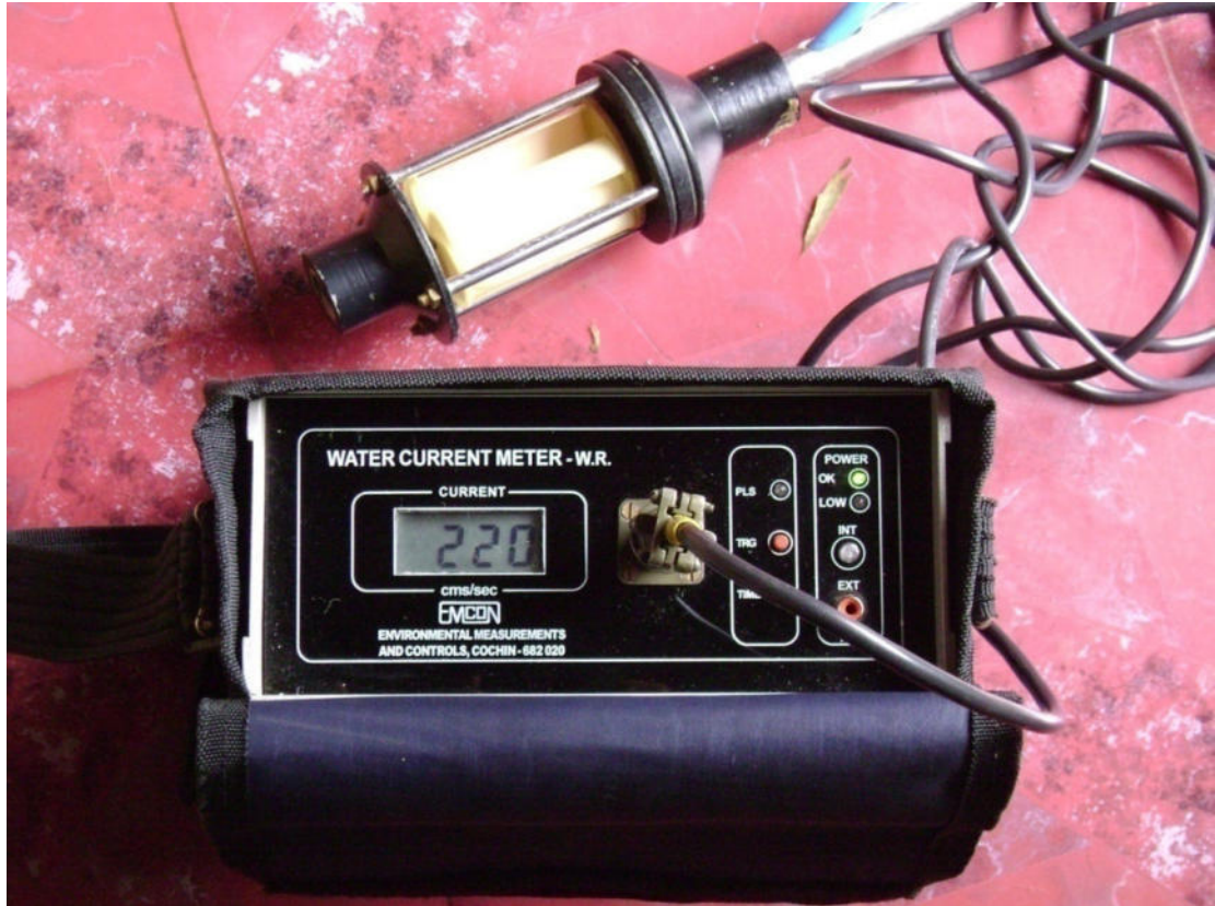
Plate 3 Wading Rod Water Current Meter
