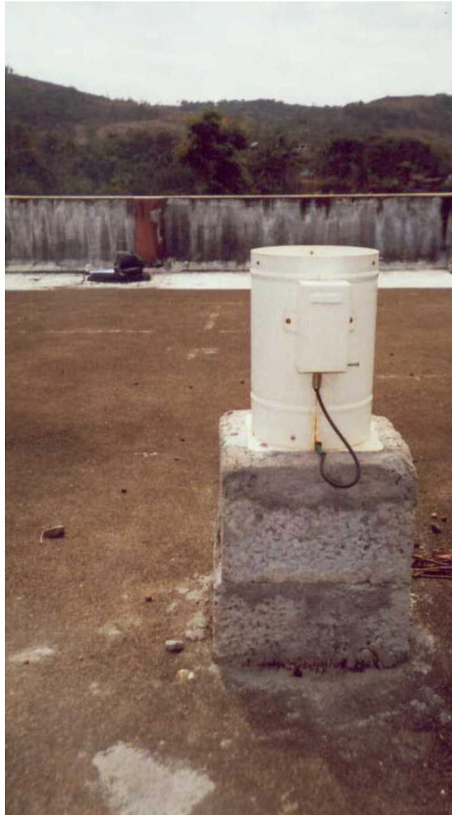
Plate 2 Electronic Raingauge installed at Pathammile
