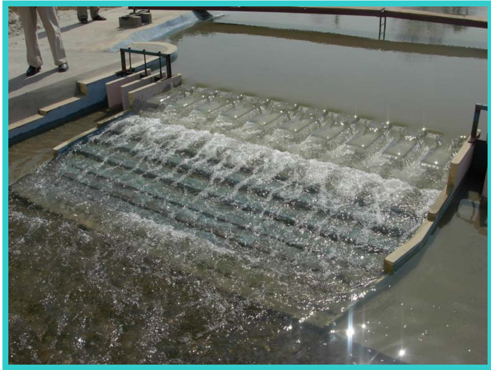
Plate No. 5.8 Running view of Piano Key Weir from d/s with under sluice gate
