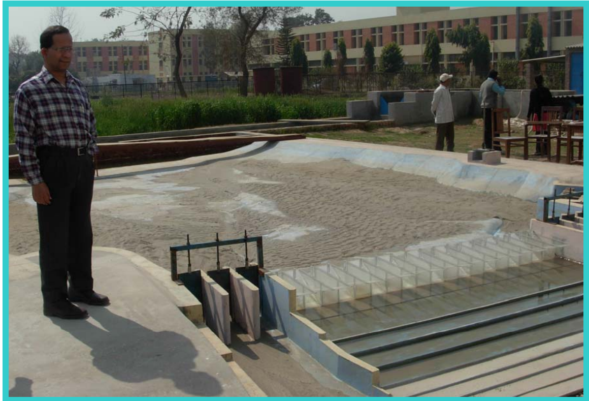
Plate No. 5.7 Pictorial view of Piano Key Weir model C 1 M 6 for comprehensive model study
