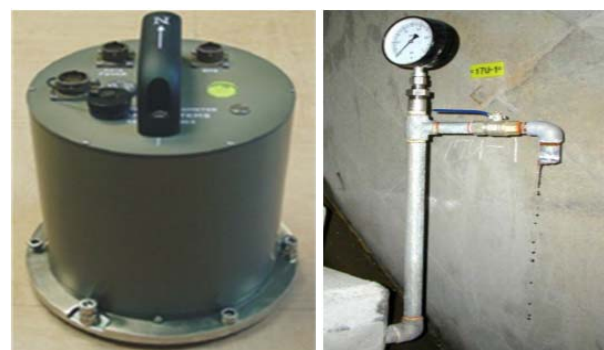
Figure 10 - Seismograph for monitoring dynamic response of dam and uplift pressure measurement
