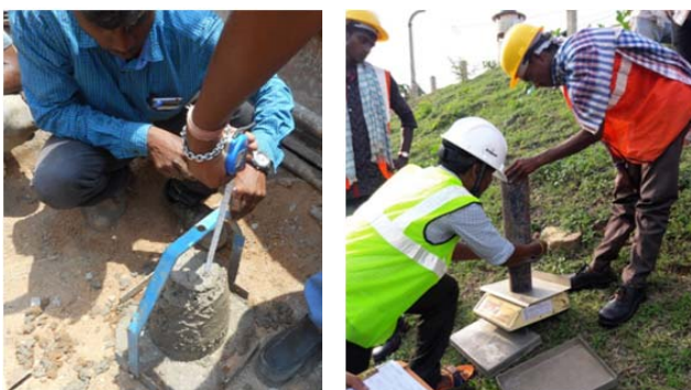
Figure 15 - Slump test at Sanamachhakandana, OWRD and Sand Replacement Test at Maithon Dam, DVC
