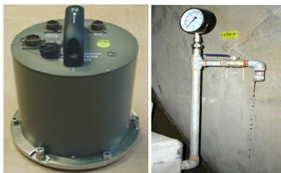
Figure 10 - Seismograph for monitoring dynamic response of dam and uplift pressure measurement
