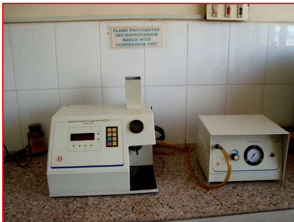
Flame photometer Level-II Laboratory at Gandhinagar
