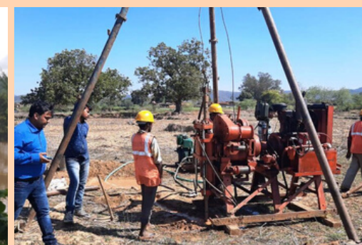
Geotechnical investigation at Barkattha Reservoir Scheme, Hazaribaag, Jharkhand
