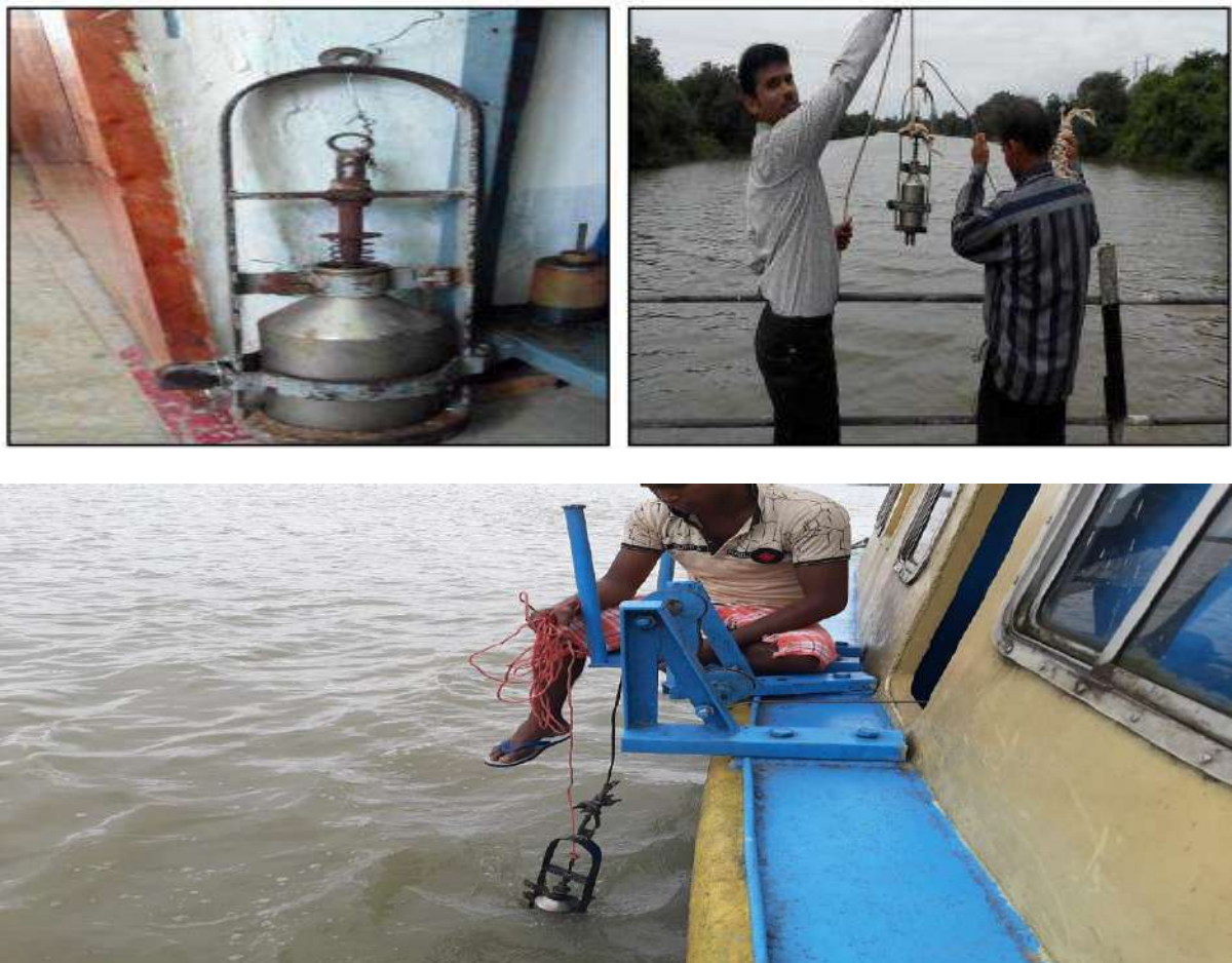
Figure 25: Measurement using Sediment Sampler
