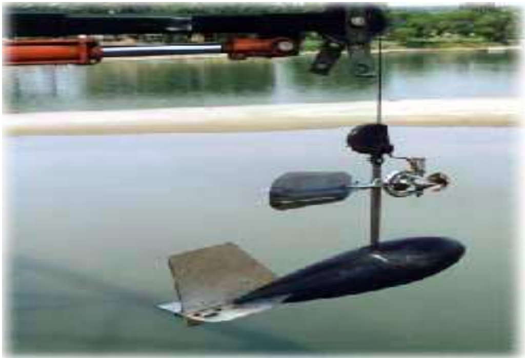
Figure 7: Current Meter While Taking Discharge Measurement
