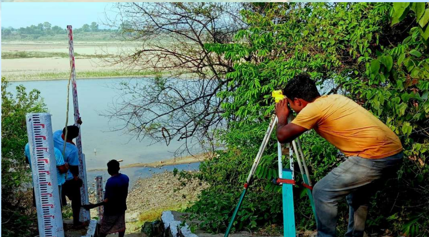
MARKING OF HIGH FLOOD LEVEL AT GOMLAI SITE ON BRAHMANI RIVER
