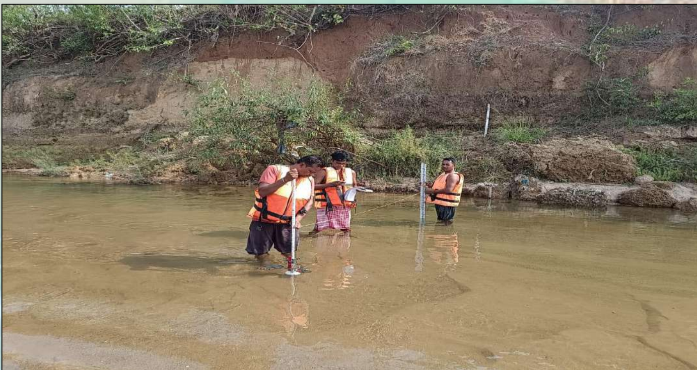
DISCHARGE MEASUREMENT WITH WADING ROD AT JARAIKELA SITE ON KOEL RIVER
