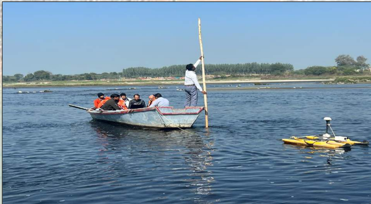
DISCHARGE MEASUREMENT WITH THE HELP OF ADCP USING BOAT AT POIYA GHAT, GDSQ
