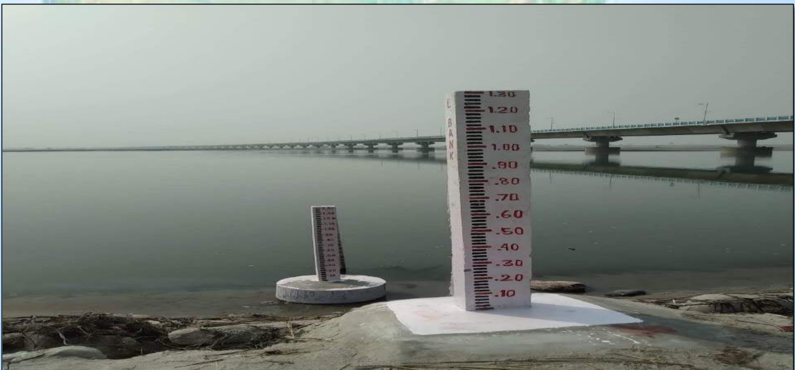
STATION GAUGE LINE AT MEKHLIGANJ R/B SITE ON TEESTA RIVER, COOCH BEHAR, WEST BENGAL
