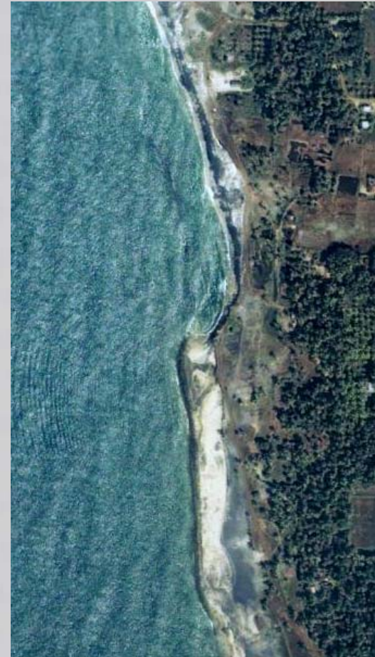
Figure 3.2 Typical end effects (terminal scour) associated with a sea wall. Note the scour which removes support from end of structure and leads to undermining at end of wall.
