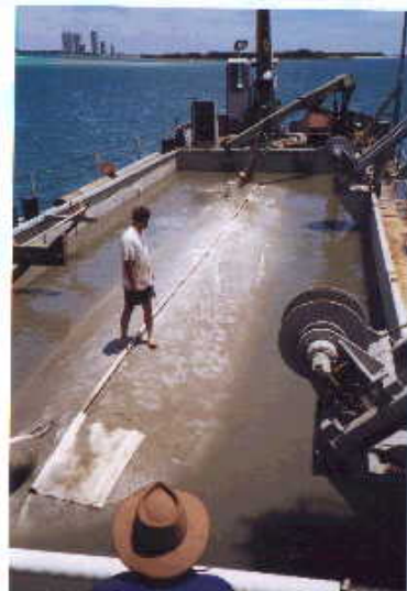
SPLIT HULL HOPPER DREDGE FILLING SANDBAG
