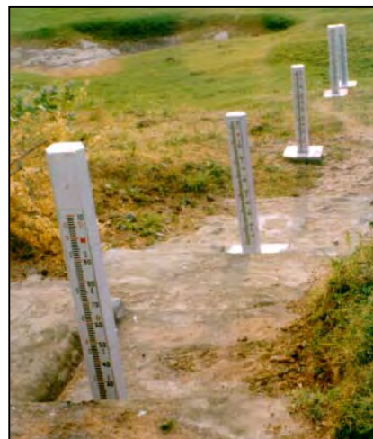
Figure 6.2a) & b): Vertical staff gauges stepped in series up a riverbank
