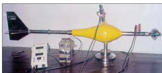
Figure 6.25(b): Propeller type current meter
