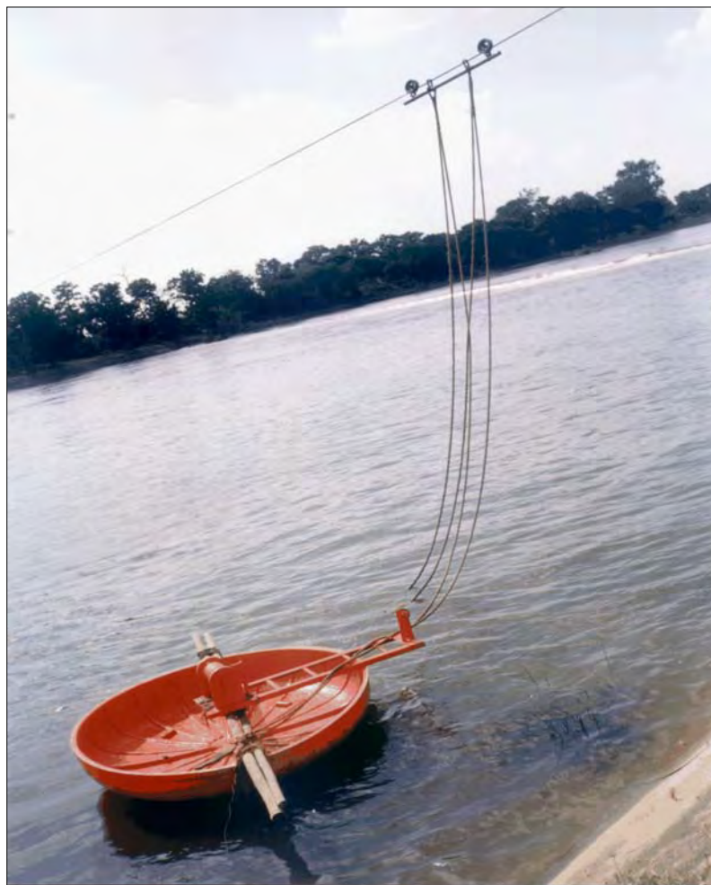
Figure 6.32: Boat gauging - boat cableway system
