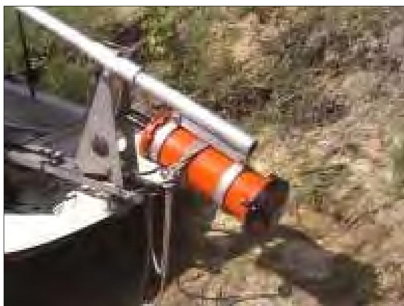
Figure 6.45(b): ADCP deployed from a boat
