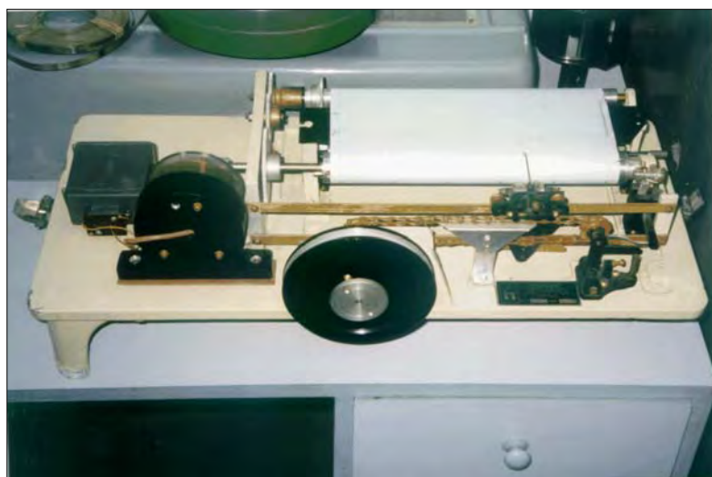
Figure 6.9: Float operated strip chart recorder
