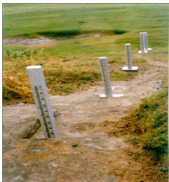
Figure 8.1: Typical Staff Gauge Installation Arrangements
