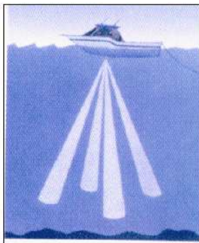
Figure 1- ADCP beams action
