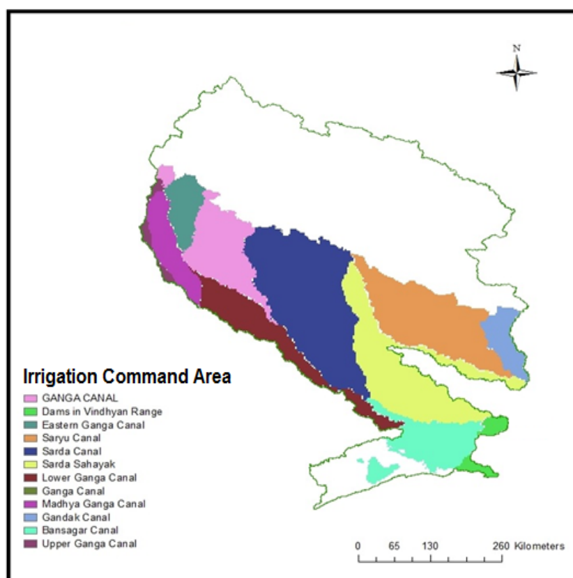
Figure 12.12 Irrigation command boundaries of Upper Ganga sub-basin
