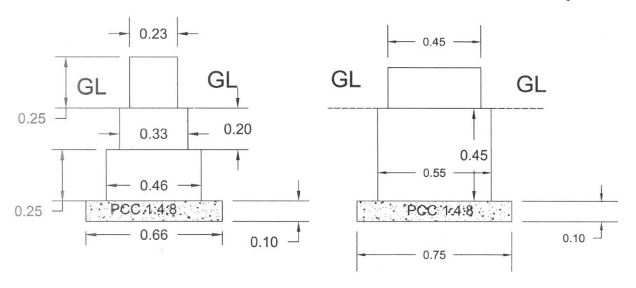
Foundation Detail of Brick & Stone Masonary Wall
