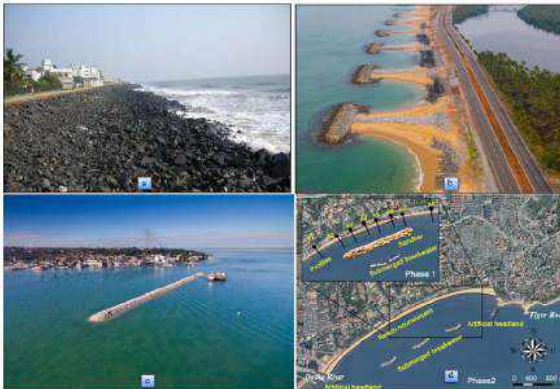
Fig. 4 Various Structural coastal protection measures (a) Sea Wall (b) Groyne field (c) Off shore breakwater (d) Artificial headland
