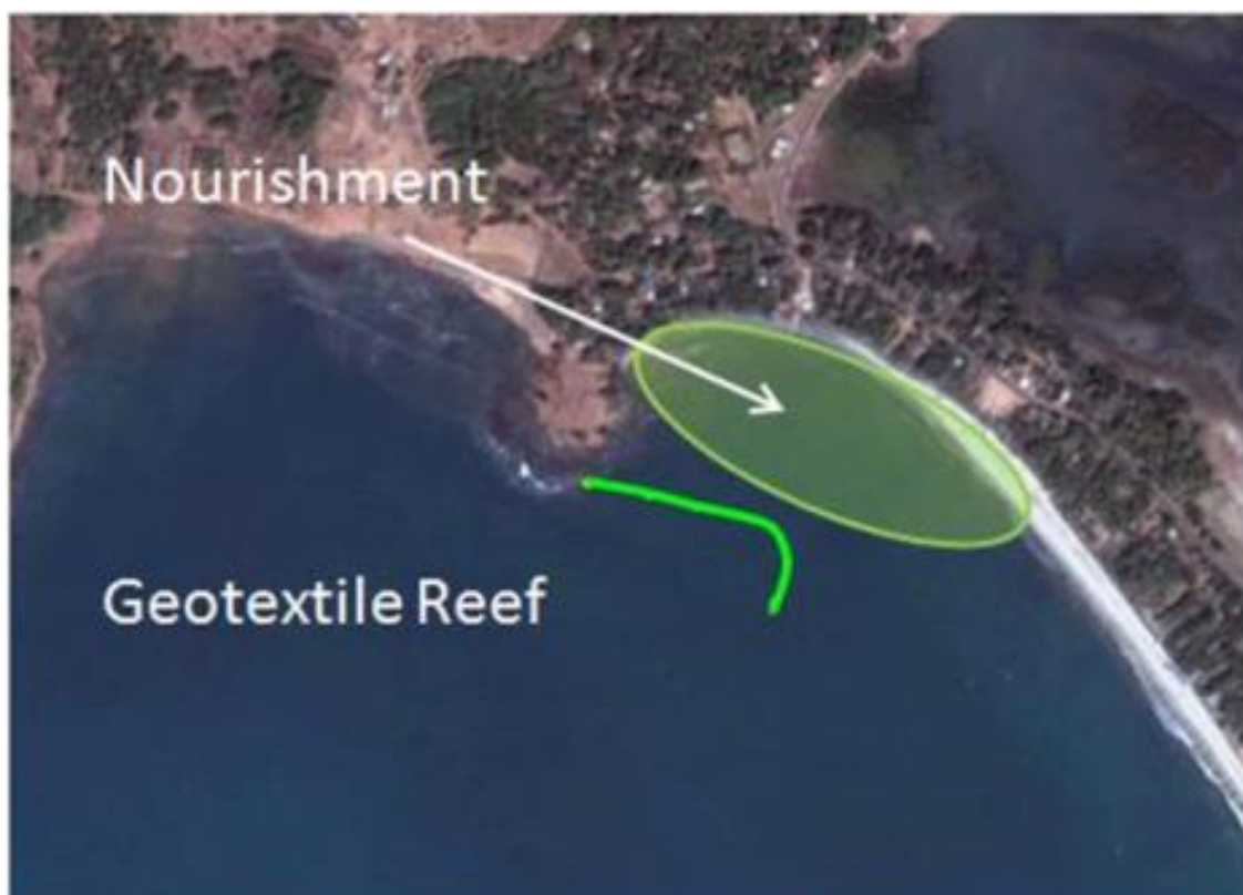
Fig 48: Solution to tackle erosion problem in Mirya Bay
