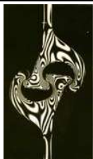
Photo-elastic studies for web sheet piles of Farakka barrage
